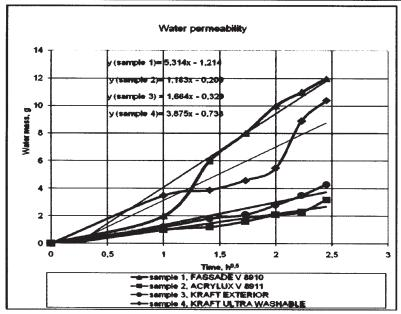
Fig. 3. The variation of the retained liquid water quantity depending on the square root of the exposure time
