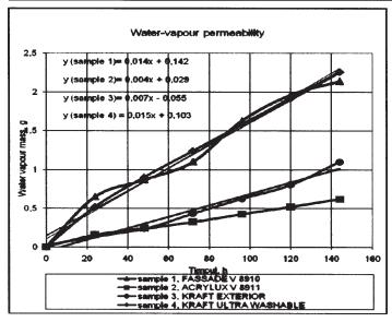
Fig. 2 The variation of the retained water-vapor quantity depending on the exposure time
