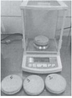
Fig.1 The weighing of test capsules before exposure to water-vapor
